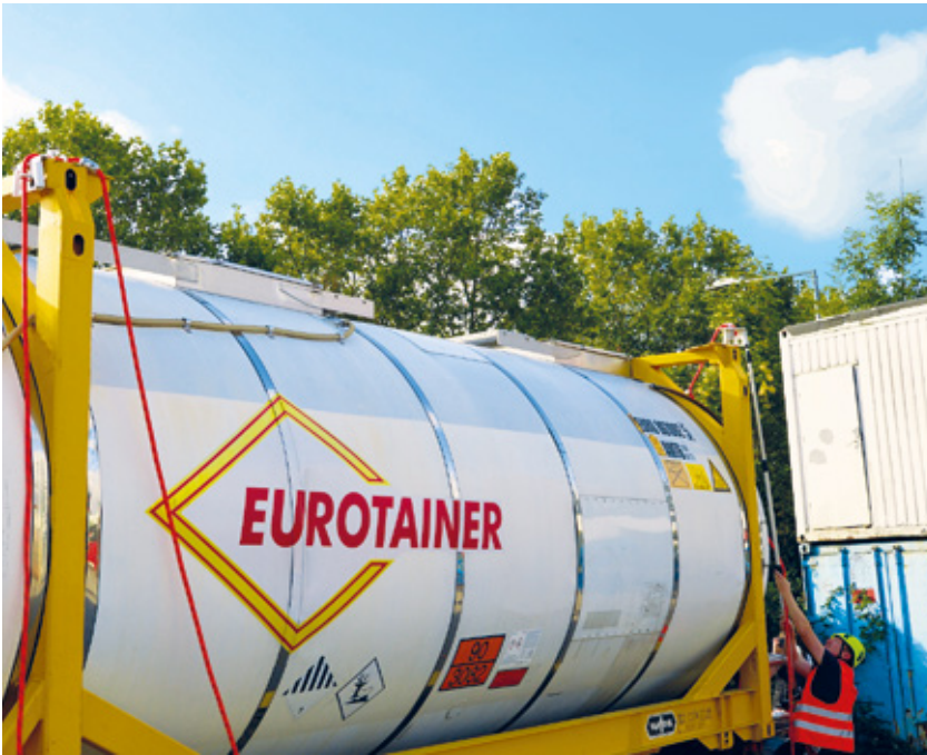
Position the corner fittings and the tension cable using the TELESCOPIC ROD
